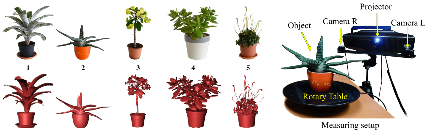
Figure 1: Images of plants (top) and corresponding point clouds (bottom). Left to right: Plant 1 ( Aechmea fasciata ), Plant 2 ( Haworthia attenuata ), Plant 3 ( Euphorbia milii ), Plant 4 ( Crassula ovata ) and Plant 5 ( Peperomia caperata ). The right side shows the setup used to scan the plants
