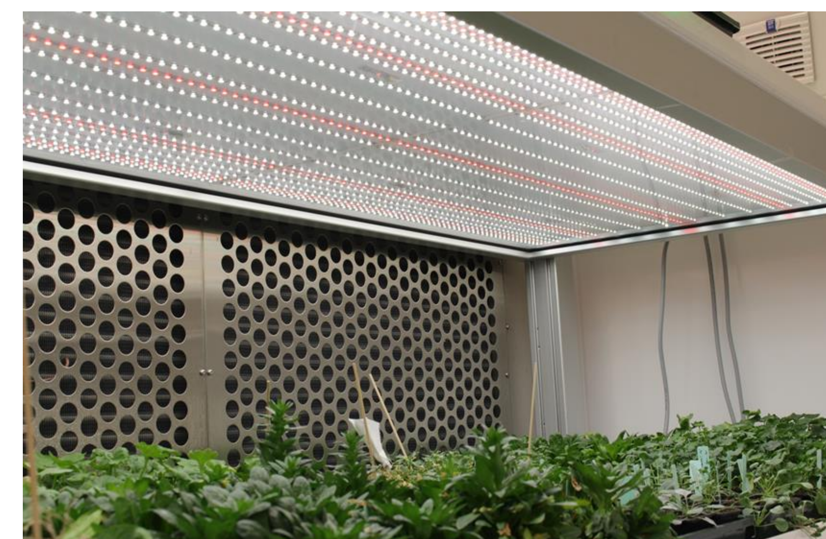
Fig. 4. White LED illumination with supplementary RED and FAR-RED LEDs (PSI) for excellent plant growth.
