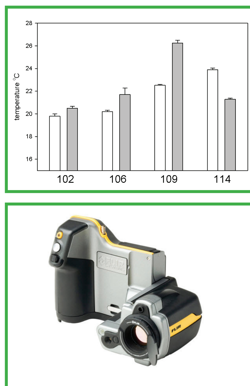
Figure 3. Leaf temperature measured for potted plants of tomato of four different genotypes : 102, 106, 109 and 114, under deficit irrigation (white bars) and under well irrigated conditions (grey bars) (up). Thermal camera used for measurements FLIR B425 (down).
