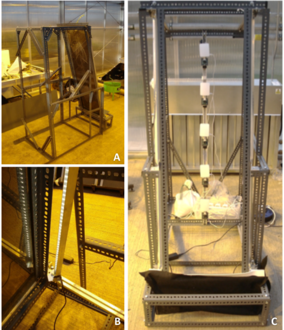
Figure 2: Imaging station. (A) Overview with of the imaging station with a mesocosm. (B) Close-up image of the LED strip. (C) Close-up of the Phenotiki sensors [14].
